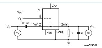
$V_{CC}$  = 4.5 V; GND = 0 V;  $V_{EE}$  = -4.5 V;  $R_L$  = 600  $\Omega$ ;  $R_S$  = 1 k $\Omega$ .
