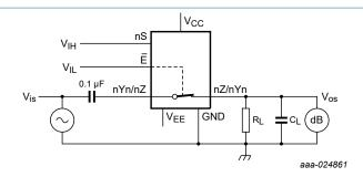
$V_{CC}$  = 4.5 V; GND = 0 V;  $V_{EE}$  = -4.5 V;  $R_L$  = 50  $\Omega$ ;  $R_S$  = 1 k $\Omega$ .
