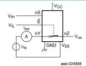
$V_{is}$  =  $V_{CC}$  and  $V_{os}$  = open
