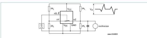
Fig. 17. Test circuit for measuring crosstalk voltage (between the digital input and the switch)
