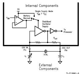
FIGURE 4. Oscillator Circuit Diagram
