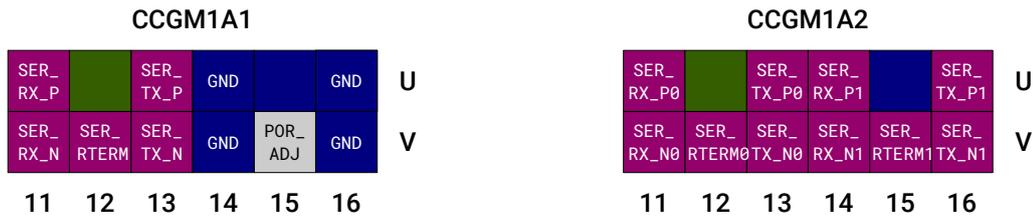
Figure 5.3: Differences between CCGM1A1 and CCGM1A2 pinout
