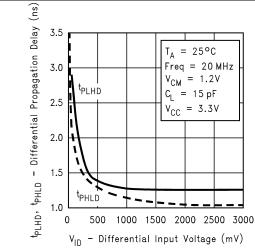
Figure 7. Differential Propagation Delay vs Differential Input Voltage
