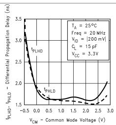
Figure 8. Differential Propagation Delay vs Common-Mode Voltage
