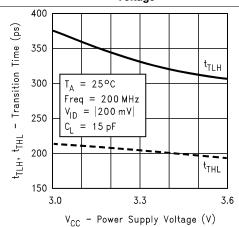
Figure 9. Transition Time vs Power Supply Voltage
