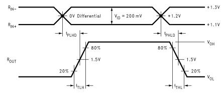
Figure 16. Receiver Propagation Delay and Transition Time Waveforms
