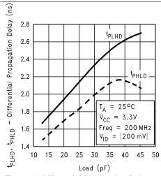
Figure 12. Differential Propagation Delay vs Load
