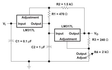
Figure 7-6. Tracking Preregulator Circuit
