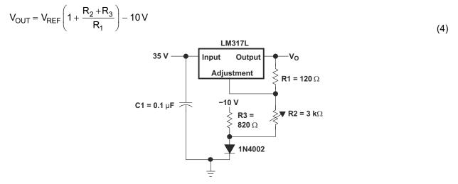
Figure 7-4. 0V to 30V Regulator Circuit
