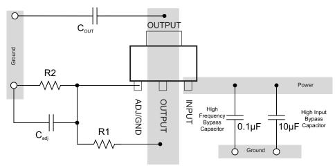
Figure 7-11. Layout Diagram
