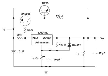
Figure 7-10. High-Current Adjustable Regulator
