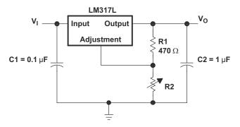
Figure 7-1. Typical Application Schematic
