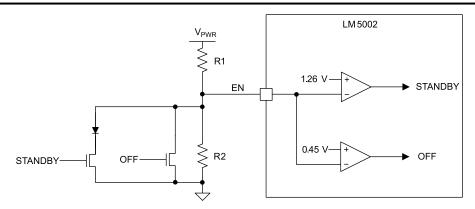
Figure 8-3. Remote Standby and Disable Control
