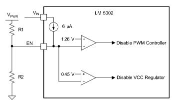
Figure 8-2. Basic EN (UVLO) Configuration
