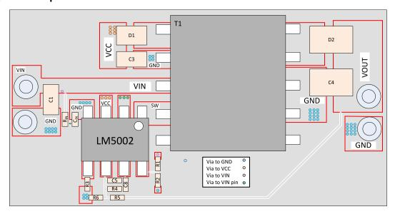
Figure 10-1. Layout Example for Figure 8-5
