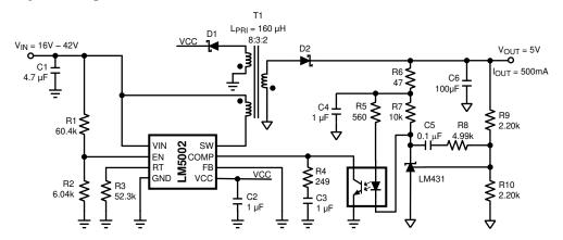
Figure 8-6. Isolated Flyback Schematic
