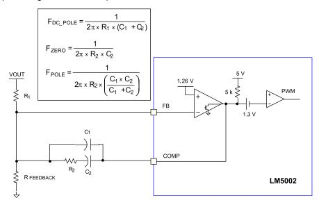
Figure 7-1. Type II Compensator
