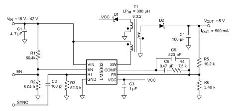
Figure 8-5. Non-Isolated Flyback Schematic
