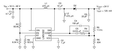
Figure 8-8. 24-V SEPIC Schematic
