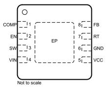
Figure 5-2. NGT Package 8-Pin WSON Top View
