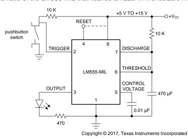
Figure 17. Schematic of Monostable Mode to Flash an LED
