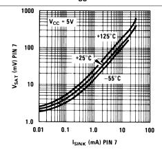
Figure 10. Discharge Transistor (Pin 7) Voltage vs. Sink Current
