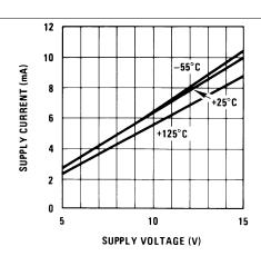
Figure 2. Supply Current vs. Supply Voltage
