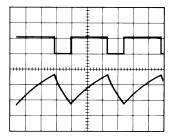
$V_{CC} = 5 V$ TIME =  $20\mu s/DIV$ .  $R_A=3.9~k\Omega$  $R_B = 3 k\Omega$
