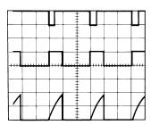
$V_{CC} = 5 V$ TIME = 0.1 ms/DIV.  $R_A = 9.1 \text{ k}\Omega$  $C = 0.01 \mu F$
