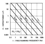
Figure 16. Free Running Frequency
