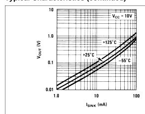
Figure 5. Low Output Voltage vs. Output Sink Current
