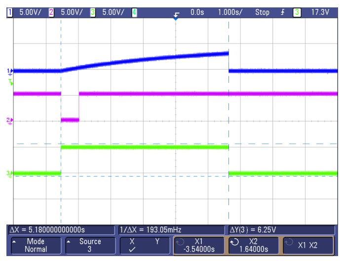
Figure 19. Trigger, Capacitor Voltage, and Output Waveforms in Monostable Mode
