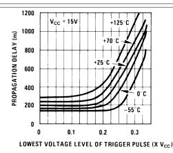
Figure 8. Output Propagation Delay vs. Voltage Level of Trigger Pulse
