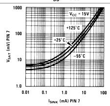
Figure 9. Discharge Transistor (Pin 7) Voltage vs. Sink Current
