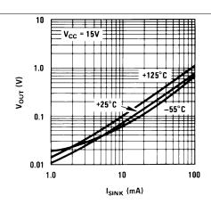
Figure 6. Low Output Voltage vs. Output Sink Current
