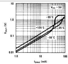
Figure 4. Low Output Voltage vs. Output Sink Current
