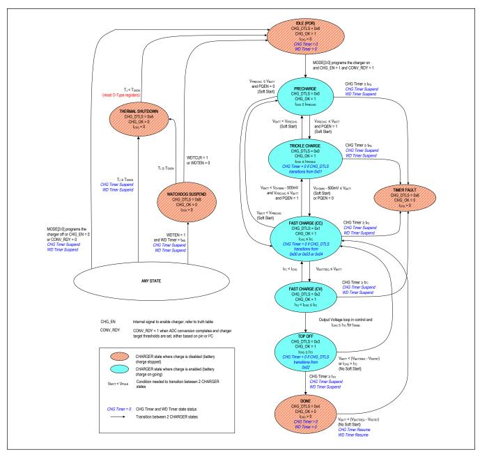
Figure 2. Charger State Diagram
