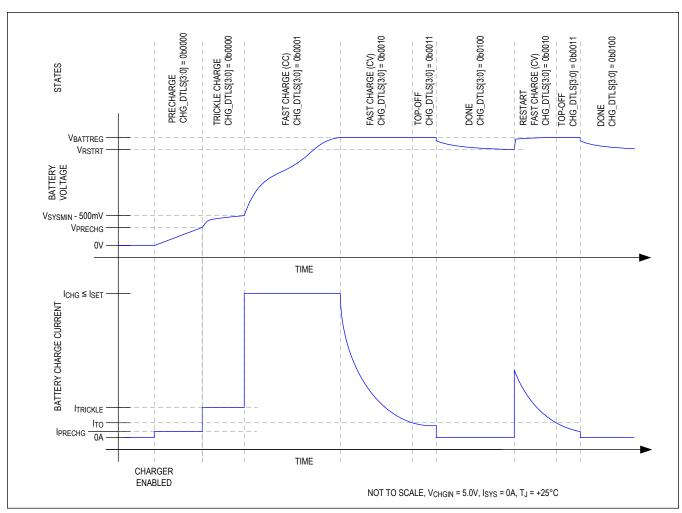
Figure 1. Li Battery Charge Profile
