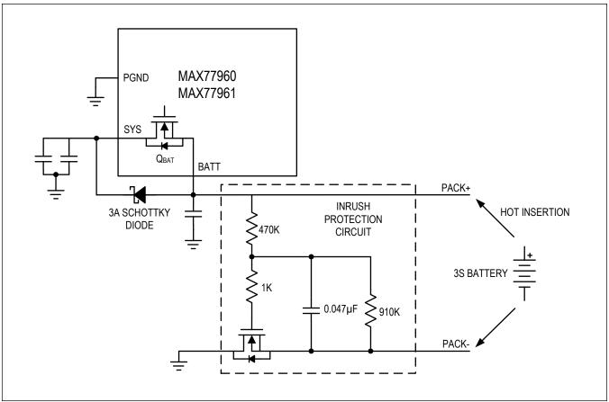
Figure 15. Battery Insertion Protection with 3S Battery
