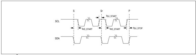
Figure 8. I<sup>2</sup>C Start Stop
