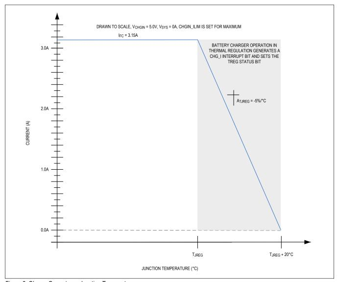
Figure 3. Charge Currents vs. Junction Temperature
