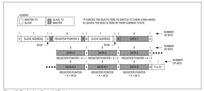
Figure 13. Reading from Sequential Registers
