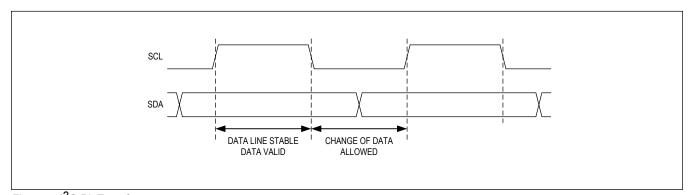
Figure 7. I<sup>2</sup>C Bit Transfer
