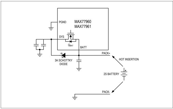
Figure 14. Battery Insertion Protection with 2S Battery
