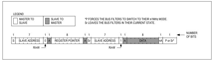
Figure 12. Reading from a Single Register
