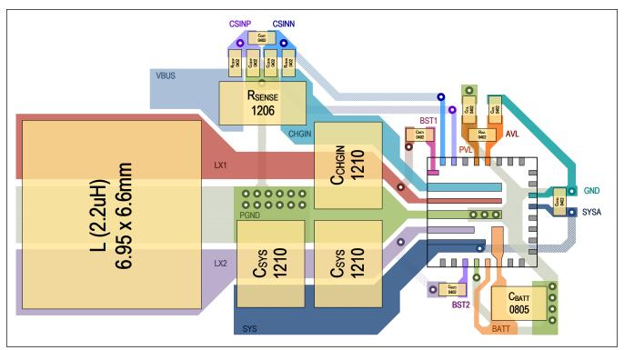
Figure 16. PCB Layout Example
