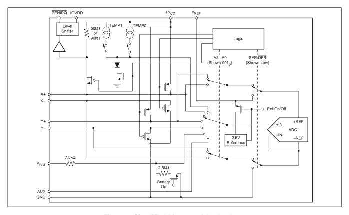
Figure 2. Simplified Diagram of Analog Input
