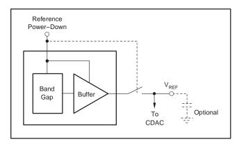
Figure 3. Simplified Diagram of the Internal Reference
