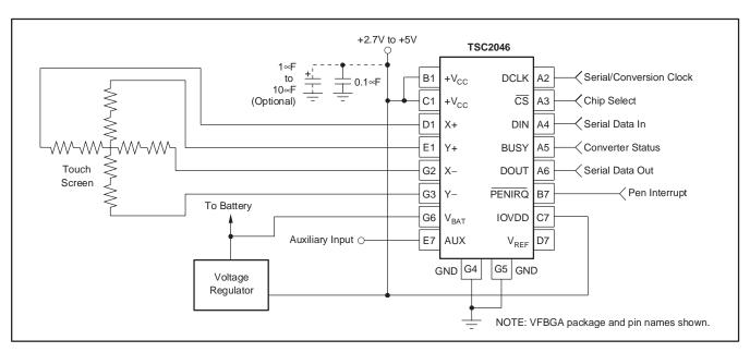
Figure 1. Basic Operation of the TSC2046
