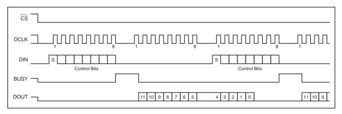
Figure 11. Conversion Timing, 16 Clocks-per-Conversion, 8-Bit Bus Interface.
