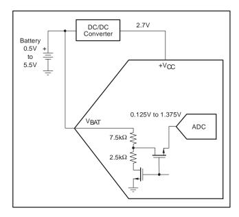
Figure 7. Battery Measurement Functional Block Diagram
