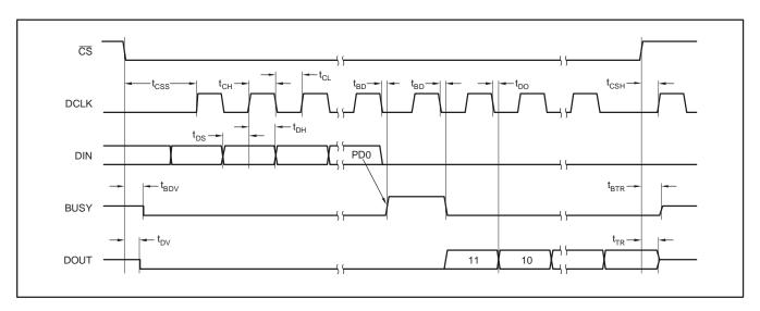
Figure 12. Detailed Timing Diagram
