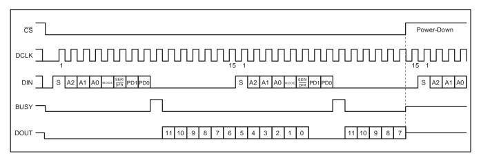
Figure 13. Maximum Conversion Rate, 15 Clocks-per-Conversion
