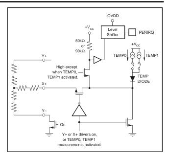
Figure 10. PENIRQ Functional Block Diagram
