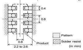
\* The excessive heat by land pads may cause deterioration at joint of products with substrate.
