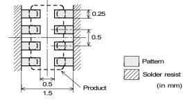
\* The excessive heat by land pads may cause deterioration at joint of products with substrate.
