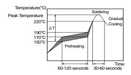
[Allowable Reflow Soldering Temperature and Time]
