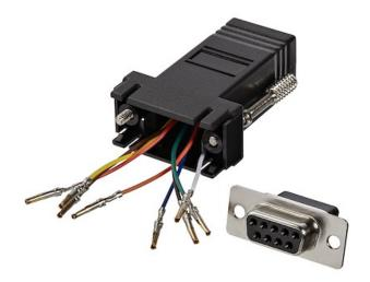
The GC98FF Modular Adapter features a DB9 female connector and an RJ45 female connector. Used for modular RS232, RS422 and RS485 connections, the adapter converts your DB9 male connection into an RJ45 female connection. The adapter allows for custom serial pin out configurations.
