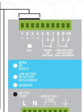
Jumper present: fast test enabled. Jumper present: fast recovery charge enabled only for size 3. Possibility to recharge the battery also when the voltage is close to zero with the maximum power of the device
