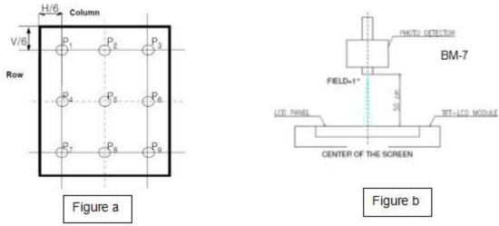
FIG.3. The definition of viewing angle
