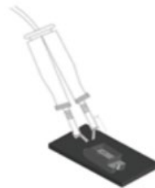
Fig2. Repairing using a double-head soldering iron
