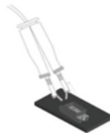
Fig2. Repairing using a double-head soldering iron
