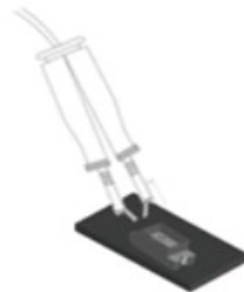
Fig2. Repairing using a double-head soldering iron
