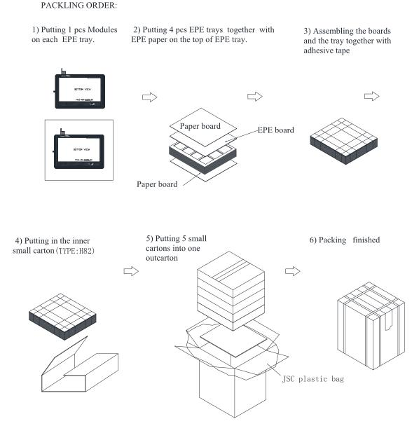
Note: 1 pcs in a tray, 4 trays in a inner carton, 5 inner cartons in a out carton, so 1x4x5=20pcs/OutcartonDimension (Small carton ): 385\*325\*87mmDimension (Out carton ): 394\*344\*470mm
