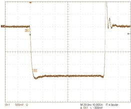
Figure: Current monitor output, scale: -10 A/Div
