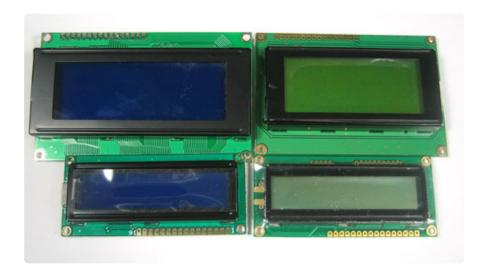
This backpack will work with any 'standard'/'classic' **character** LCD. It does not work with **graphic** LCDs. Character LCDs come in sizes ranging from 8x1 (8 characters, one line) to 40x4 (40 characters, four lines). The backpack will also only fit LCDs that have a single line of pins at the top, not the ones that have a 2x10 or 2x8 connector on the side. Those are much rarer these days but just keep a look out for that!
