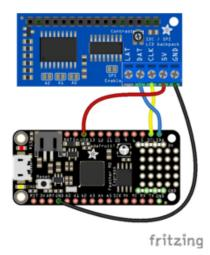
Board VUSB to backpack 5V (remember using the VUSB output on a Feather means it must be connected to a 5V USB power source like your computer or a battery pack! You can alternatively use the 3.3V output of the Feather but it might not be enough to power the LCD.)
