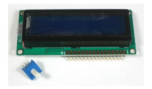
The easiest way we know of doing this is sticking the header into a breadboard and then sitting the LCD on top while soldering. this keeps it steady.
