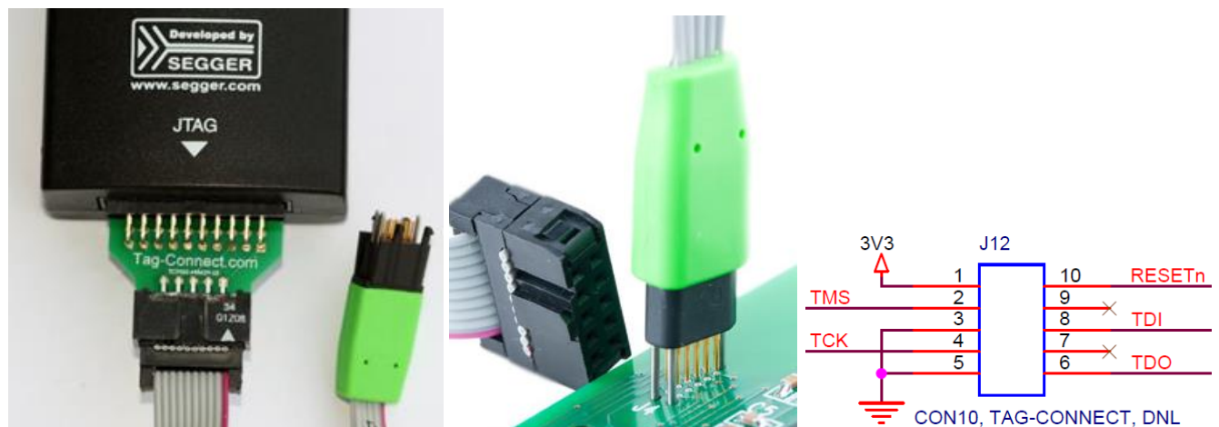
Figure 4 – Tag-Connect JTAG adapter, cables, and pinout for 10-pin TC2050
