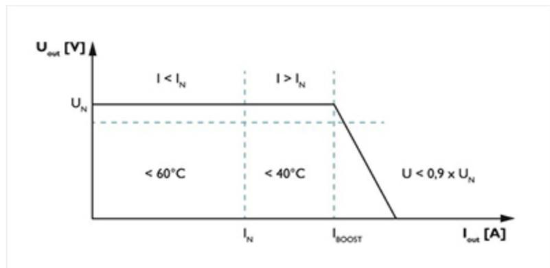
capacitive loads have to be absorbed without voltage dips. With the QUINT Power Boost function a static boost will continuously provide up to 125% of the nominal current. In addition, you can use the dynamic boost to supply 200% of the nominal current for 5 seconds when starting up heavy loads.
