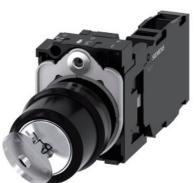
RONIS key-operated switch, 22 mm, round, plastic, lock number SB30, with 2 keys, 2 switch positions O-I, latching, 10:30h/13:30h, key removal O+I, with holder, 1 NO+1 NC, screw terminal, possible special locks: SB31, 421, 455, with laser labeling, inscription or symbol Customer-specific selection with SIRIUS ACT configurator (CIN)
