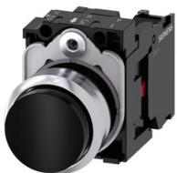
Pushbutton, 22 mm, round, metal, shiny, black, pushbutton, raised, momentary contact type, with holder, 1 NC, screw terminal, Z=20-unit packaging
