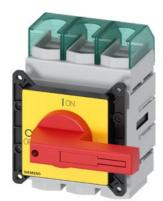
SENTRON, Molded case switch 3LD5 UL, Emergency switching-off, 3-pole, certified according to UL489 UL60947-4-1 and IEC60947-3, UL: 150A, SCCR 50kA at 480VAC, Operating power at 480VAC 3-phase: 100hp, IEC: 160A, Operating power at AC-23A at 400V: 75kW, front-mounted, rotary operating mechanism, red/yellow, 4-hole mounting of the handle, incl. terminal covers for the infeed side
