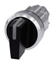
Illuminable selector switch, 22 mm, round, metal shiny, black, Selector switch short, 3 switch positions I>O<II, momentary contact type, actuating angle  $2x45^\circ$ , 10:30h/12h/13:30h
