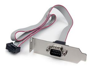
The PLATE9M16LP (16 inch/ 0.4 m) Low Profile Serial Plate adds a DB9 serial port to the rear panel of a small form factor/low profile computer, connecting to an IDC10 header connector on the motherboard.
