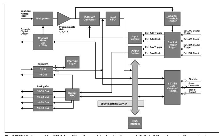
The DT9834 Series provides USB 2.0 multifunction modules for simultaneous A/D, D/A, DIO, and counter/timer subsystem operation. This detailed block diagram shows the relationship of each subsystem and the control signals used in the series. For flexible, cost-effective solutions, you can choose the number of analog I/O channels as well as the packaging configuration that suits your application.
