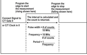
Programmable edges allow you to use counter/timers to measure the pulse width, frequency, and period of signal.
