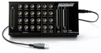
DT9834 Series modules are available in two configurations: BNC connection box and OEM embedded version.
