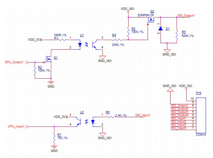
Isolated GPIO reduced schematic
