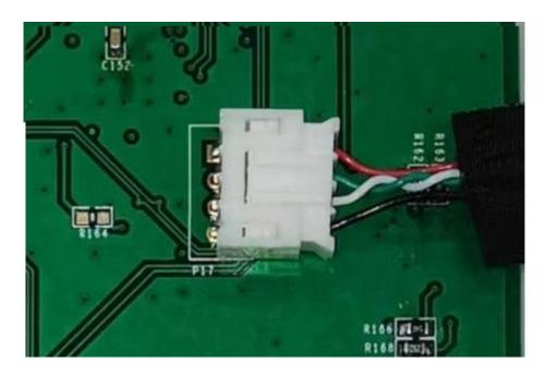
Figure 614: Capacitive Touch Connector
