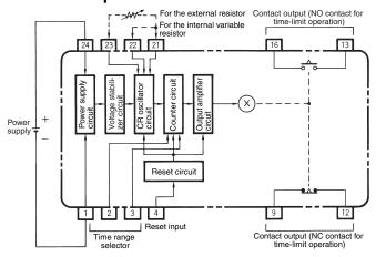
The voltage across the H3FA-SA and -SB (solid-state output loads) is the load input voltage minus the residual voltage when the transistor turns ON.
