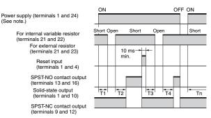
**Note: 1.** Control output is provided when the set time has elapsed  $(T_1 + T_2 \text{ or } T_3 + T_4)$ .
