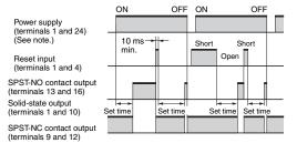
Note: When using a 12/24 V DC-operated model with a 12 V DC power supply, short terminals 13 and 15.
