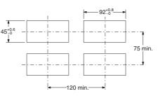
Note: The values above are recommended values. Do not group-mount the meters at intervals less than the recommended ones.
