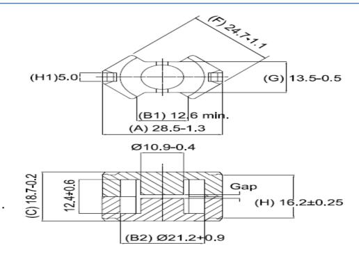
Remarks: Value of "G" is Zero (0) for Un-Gapped Cores, for Gapped Cores the value of "G" varies as per the Gap/AL value
