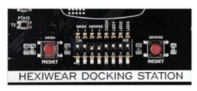
There is a row of 8 configuration switches right under the Hexiwear connector. Switches 1-5 are for setting up the OpenSDA programmer/debugger to connect either to the K64 MCU or the KW4x BLE MCU.
