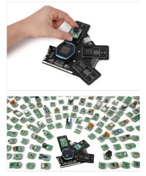
The click board eco-system vastly enhances Hexiwear's potential as a development tool. Hundreds of sensors, actuators, transceivers, displays, ports, encoders and interfaces are available on click boards – add-on boards with a standardized connector and form factor.
