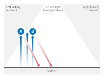
• In order to recognize two objects close to each other (A and B), a separation must allow at least one emitterreceiver channel (~10 mm) to pass freely between them. Otherwise, the two objects will be reported as one large object.
