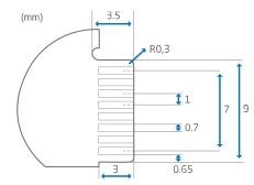
The contact pads are placed on the backside of the Touch Sensor PCBA.
