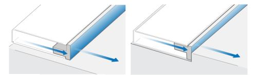
When integrating zForce AIR Touch Sensor into a host system make sure not to interfere with the light path. For horizontal integration, the opening for the sensors light path must be *minimum 1.4 mm*.
