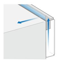
To make sure not to interfere with the sensor light path, opening must be *minimum 1.6 mm*. If host system have large tolerances, opening must be adjusted to always be minimum 1.6 mm. Also note that it is not allowed to mount, glue or in any other way affect the sensors optical surfaces since it will affect the performance. This applies to both the sensors visible optical surface and also the built-in optical surface A (mirror surface).
