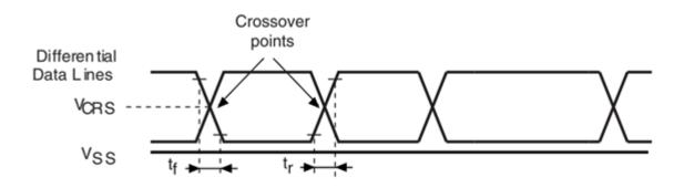
USB full speed timings: definition of data signal rise and fall time.
