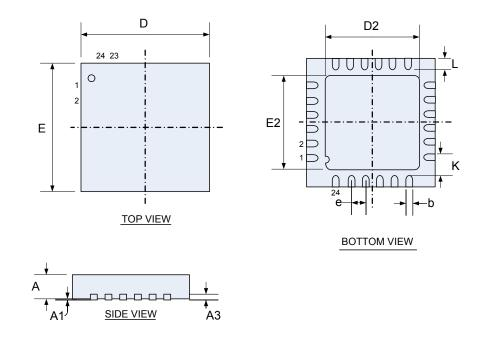
Figure 76. QFN24 pin 4×4mm
