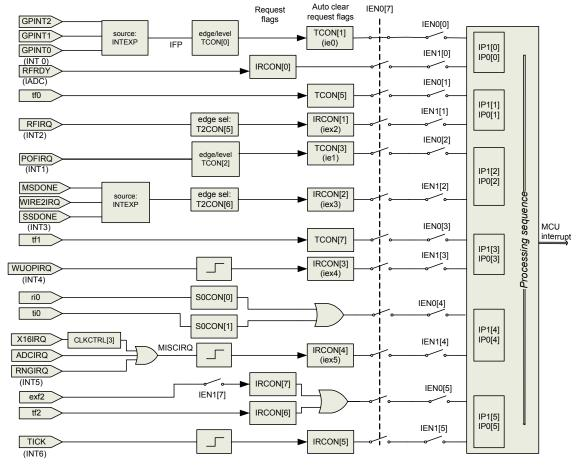
Figure 46. Block diagram of interrupt structure
