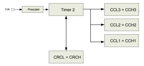
Figure 44. Timer 2 block diagram
