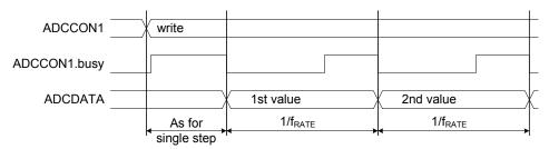
Figure 72. Timing diagram for continuous conversion
