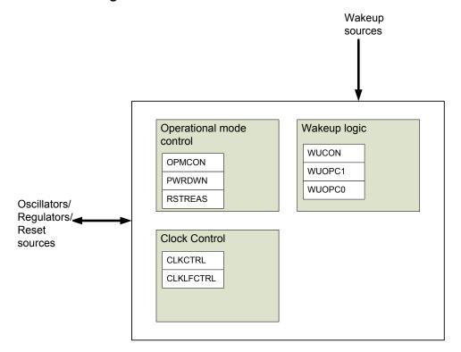
Figure 48. Block diagram of power and clock management
