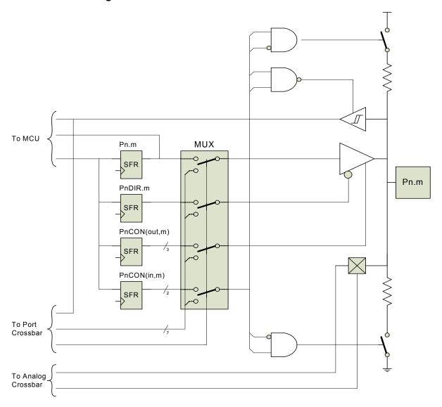
Figure 59. IO pin circuitry block diagram
