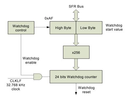
Figure 47. Watchdog block diagram
