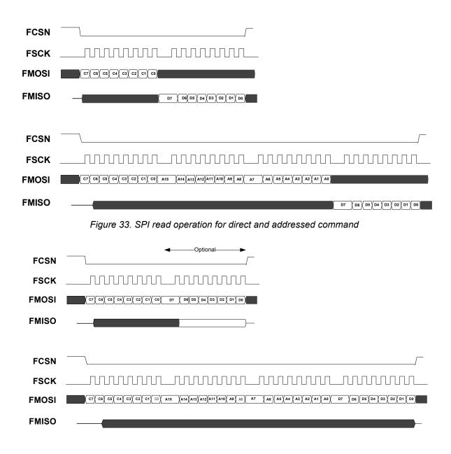
Figure 34. SPI write operations for direct and addressed commands
