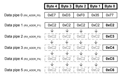
Figure 15. Addressing data pipes 0-5
