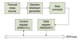
Figure 58. Block diagram of RNG
