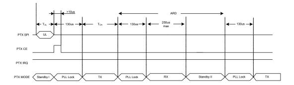
Figure 19. Timing of Enhanced ShockBurst™ when the first ACK packet is lost (2Mbps)
