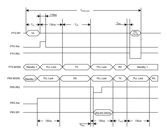
Figure 18. Timing of Enhanced ShockBurst™ for one packet upload (2 Mbps)
