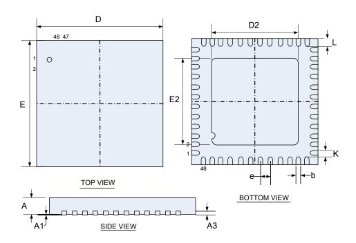
Figure 78. QFN48 pin 7×7mm
