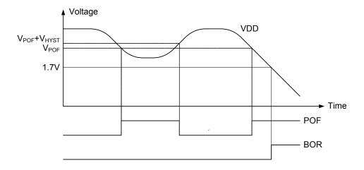
Figure 53. Power-fail comparator
