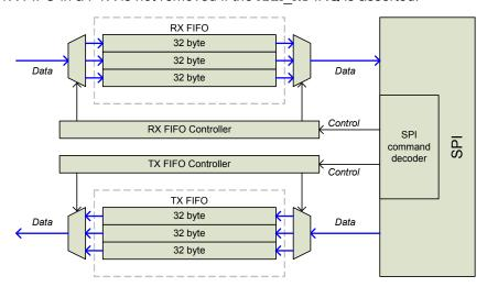
Figure 28. FIFO (RX and TX) block diagram
