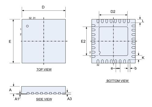
Figure 77. QFN32 pin 5×5mm
