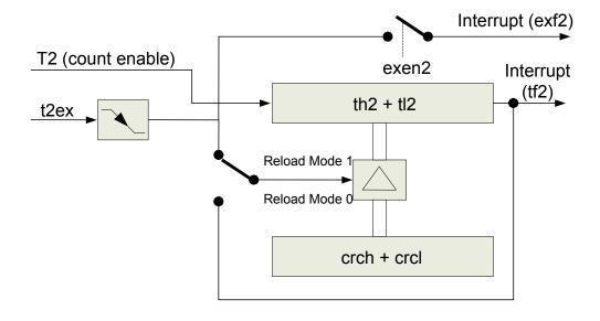
Figure 45. Timer 2 in Reload Mode
