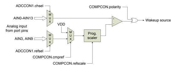
Figure 74. Block diagram of analog comparator
