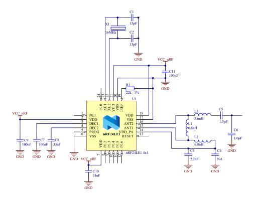
Figure 81. nRF24LE1, 4×4mm QFN24 schematic
