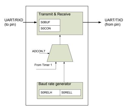
Figure 65. Block diagram of serial port
