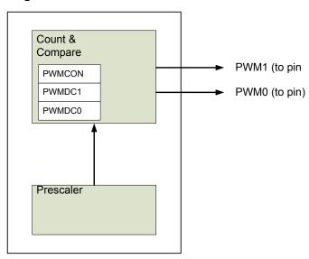
Figure 75. Block diagram of PWM
