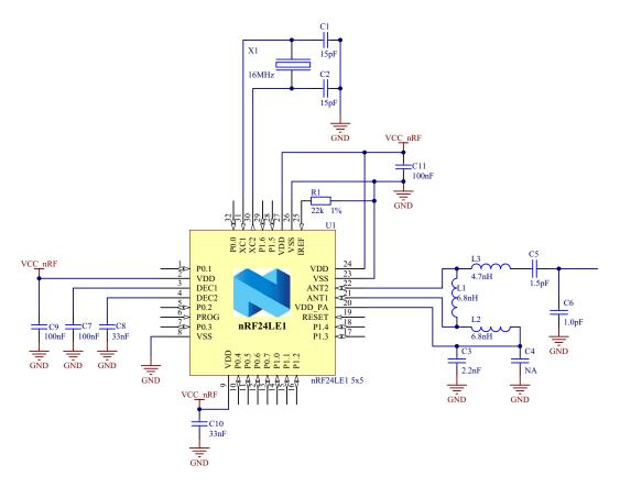
Figure 80. nRF24LE1, 5×5mm QFN32 schematic
