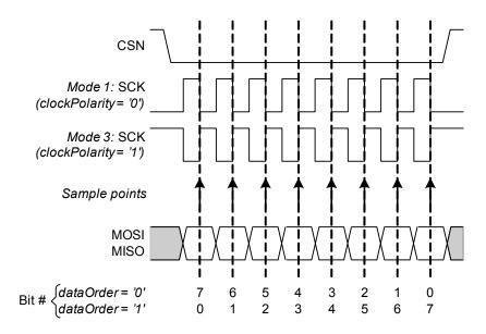
Figure 63. SPI Modes 1 and 3: clockPhase = '1'. One byte transmission.
