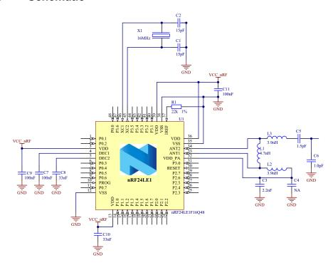
Figure 79. nRF24LE1, 7×7mm QFN48 schematic
