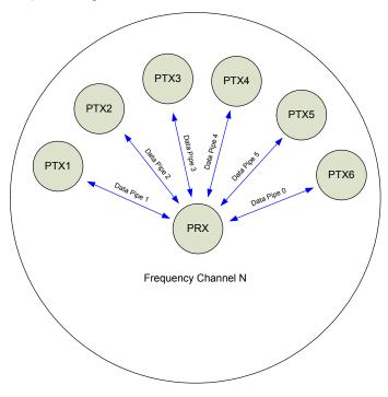
Figure 14. PRX using MultiCeiver™
