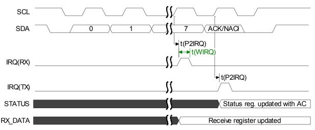
Figure 68. Interrupt request timing towards MCU
