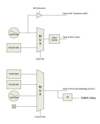
Figure 49. nRF24LE1 clock system
