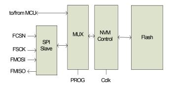
Figure 31. nRF24LE1 Flash block diagram
