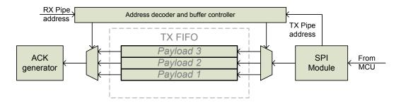
Figure 11. TX FIFO (PRX) with pending payloads
