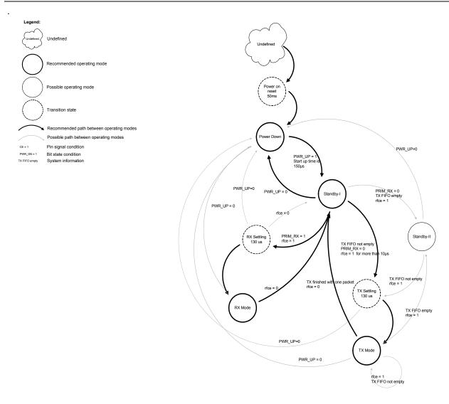
Figure 6. Radio control state diagram
