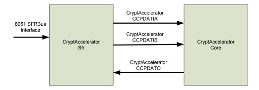
Figure 57. Encryption/decryption accelerator
