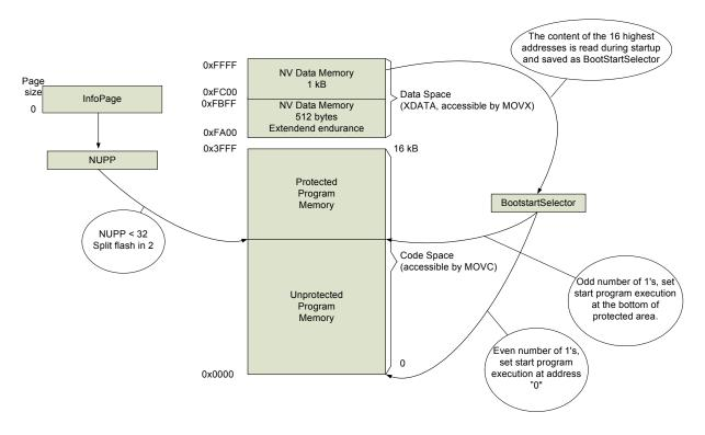
Figure 32. Flash main block protected area
