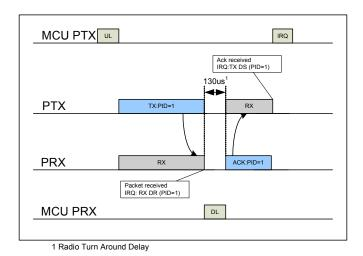
Figure 20. TX/RX cycles with ACK and the according interrupts
