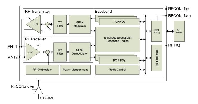
Figure 5. RF transceiver block diagram
