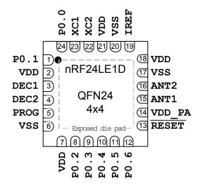
Figure 2. nRF24LE1D pin assignment (top view) for a QFN24 4×4 mm package
