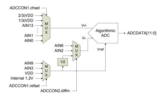
Figure 70. Block diagram of ADC
