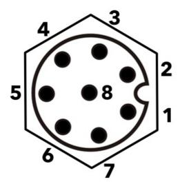
View as looking into the M8 connector on the outside of the enclosure.
