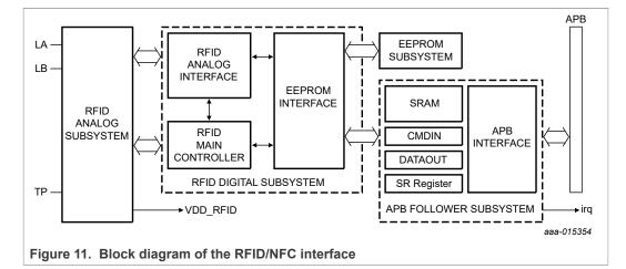
The CMDIN, DATAOUT, status register (SR), and SRAM are mapped in the user memory space of the RFID core. The RFID READ and WRITE commands allow wireless communication to this shared memory.
