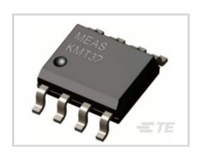
Position Sensor Product Type: Magnetic Angle Sensor
